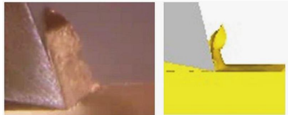
Figure 3. Comparison of chip formation between experiment and simulation
