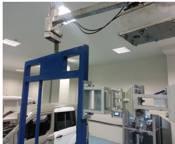
Figure 3. Hinge durability test bench
