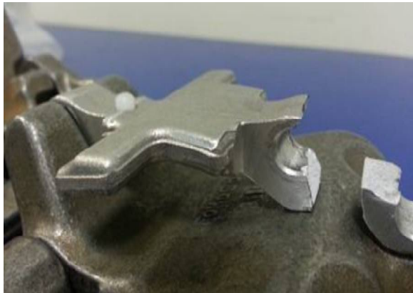
Figure 11. Failed aluminum link after durability test
