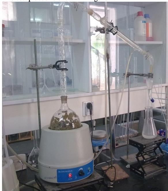
Fig.1 Installation of hydrodistillation (Clevenger apparatus) - [10]
