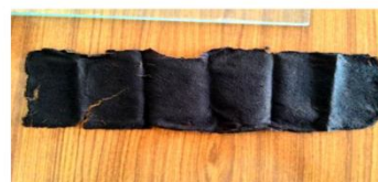
Final bioplastic film after drying.
