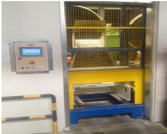
Fig. 3. Control unit of the automation system
